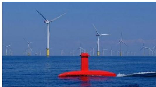
Specific locations of interest were identified within the wind farm environment to provide a direct comparison with conventional survey methodologies. Fitted with a Teledyne RESON Seabat IDH T50 multibeam echosounder, the system was able to acquire unprecedentedly clean bathymetry at speeds greater than eight knots, remaining on the intended survey line in cross-tides in excess of 1.5 knots.
