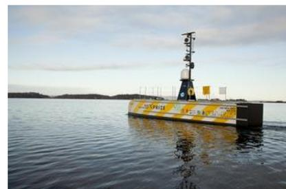
Sea-Kit can carry a deployable and retrievable payload of up to 2.5 tons and is anticipated to make seafloor mapping safer and more efficient. It uses Kongsberg Maritime's K-MATE, an autonomous control engine that is also being deployed for the fully electric, autonomous container feeder Yara Birkeland.
